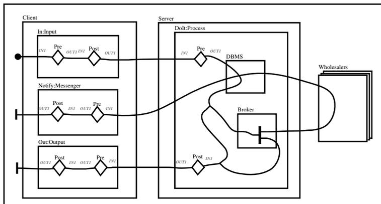
Figure 7: Extending the Client-Server system with broker functionality.
