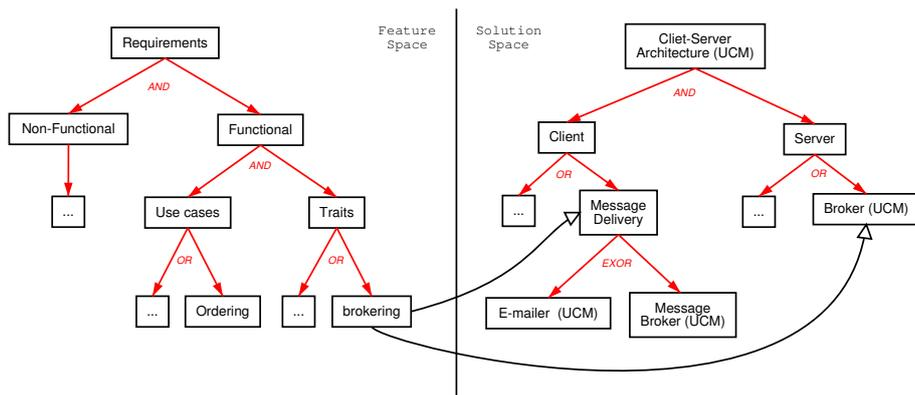
Figure 8: Feature-Solution graph for the Client-Server system.
