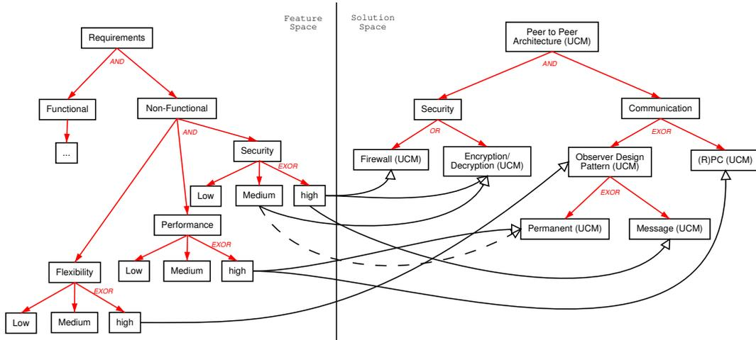
Figure 4: Feature-Solution graph for peer to peer communication.
