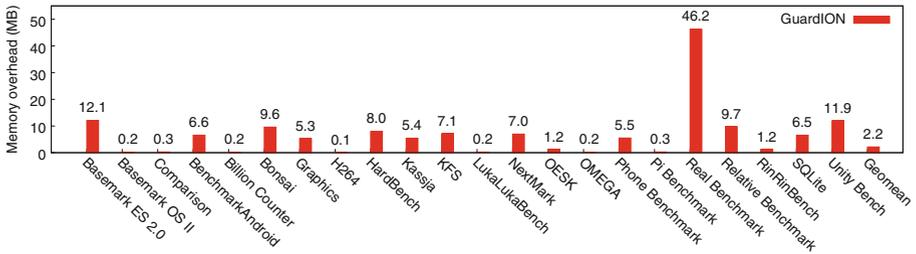
**Fig. 6.** Memory overhead of DMA isolation with GUARDION. The numbers show the overhead in MB. The last column reports the geometric mean of these results (2.2 MB), which indicates that the memory overhead is, in the general case, negligible.
