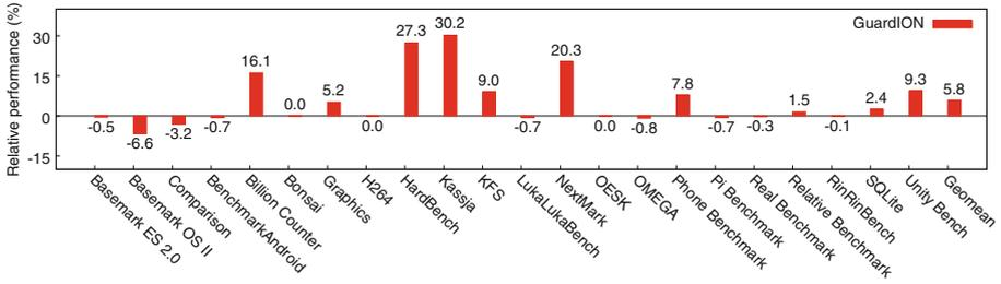
**Fig. 5.** Performance results of applying GUARDION. The numbers show the relative improvement (positive number) or degradation (negative number) of the performance according to each benchmark app. The last column reports the geometric mean of these results (5.8%), which shows that the performance generally increases.
