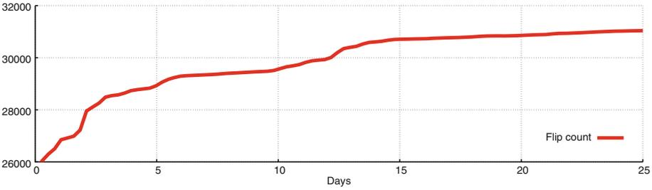
**Fig. 1.** Number of unique bit flips found while repeatedly hammering the same 4 MB chunk using double-sided Rowhammer on a Nexus 5 over a time-period of 25 days. Results were obtained by using Drammer’s source code [3].
