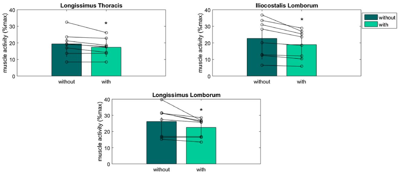
**Fig. 8** Muscle activity of the back muscles with and without the exoskeleton, averaged over all participants.  $N=8$ . Error bars indicate standard deviations. Black lines indicate individual responses. \*Sig-
