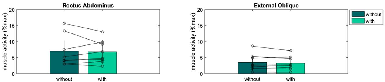
**Fig. 9** Muscle activity of the abdominal muscles with and without the exoskeleton, averaged over all participants.  $N=8$ . Error bars indicate standard deviations. Black lines indicate individual responses
