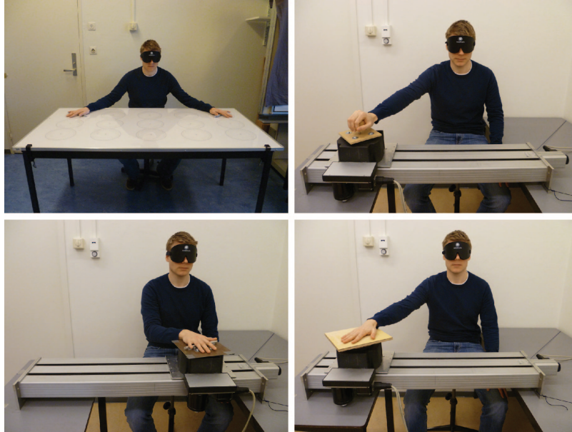
Fig. 1. Participant in the various experimental conditions. Top left: “parallel”; bottom left: “bar”; top right: “sphere”; bottom right: “plane”. In “bar” the position of the stimulus is in its leftmost position, and in “sphere” and “plane” in the rightmost position.
