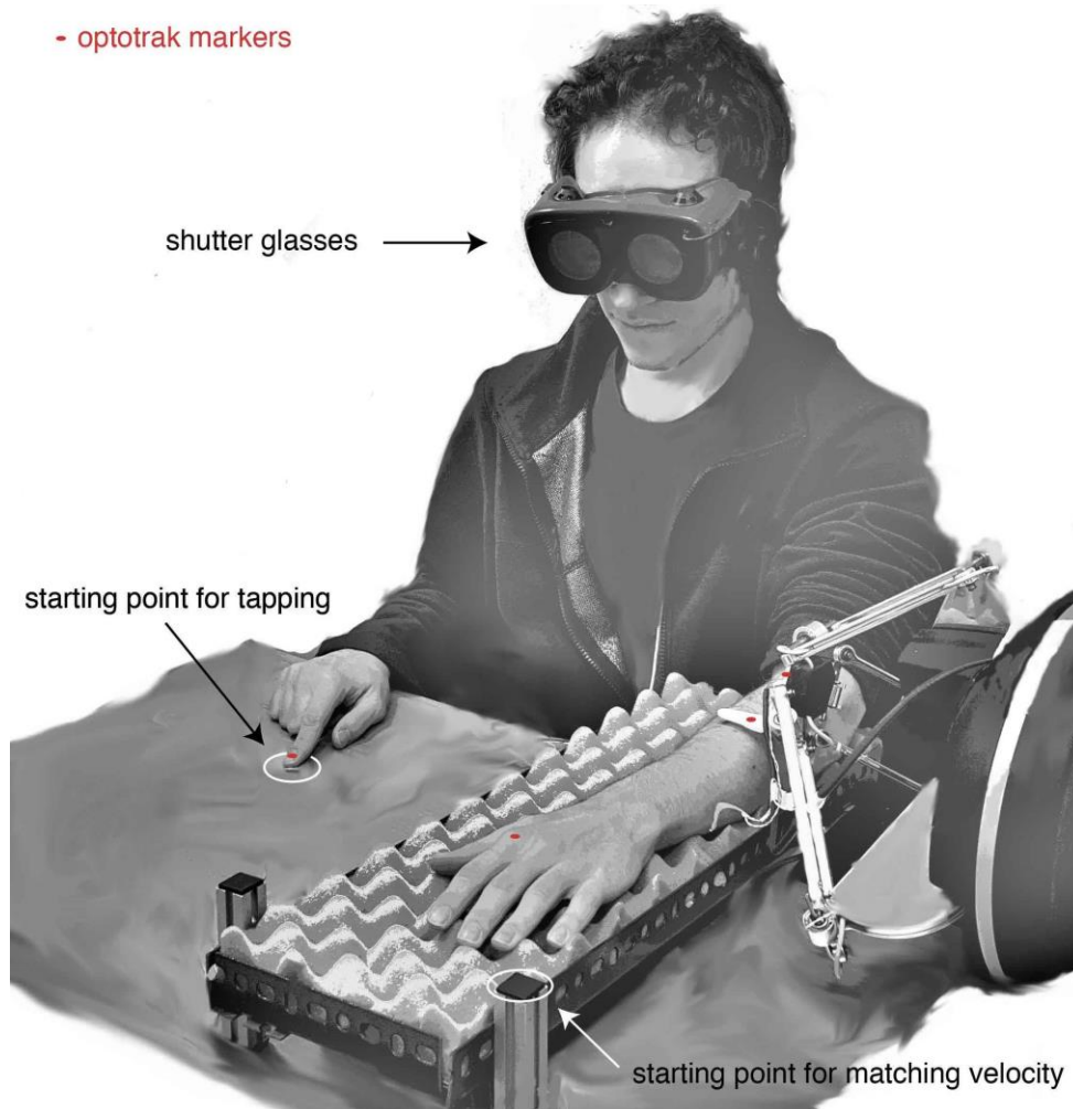
Figure 5.1. The experimental setup. Red dots indicate the position of the Optotrak markers, and white circles indicate the two starting points for the finger, one for the tapping movements of the Position and Interception experiments and the other for the movements in the Velocity experiment.
