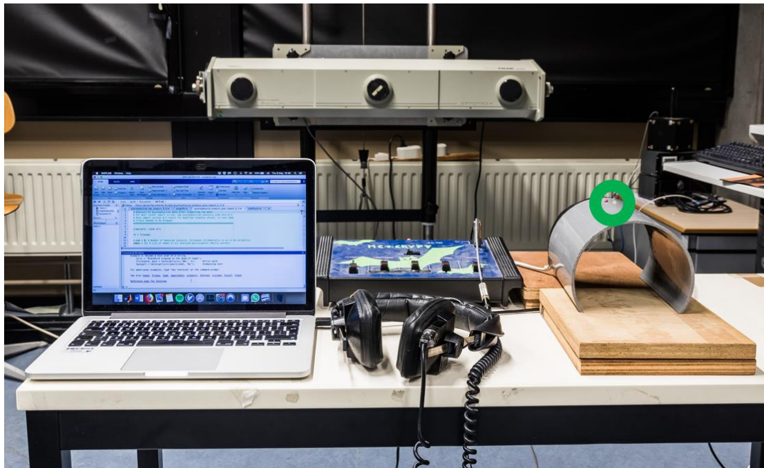
Figure 3.1. Experimental setup. Room and laptop screen are well lit for clarity. Participants placed their hand inside the pipe on the right. The green LED atop the pipe (the LED on the right within the area indicated by the green circle; the other, red LED was not used in this study) provided the visual stimuli.
