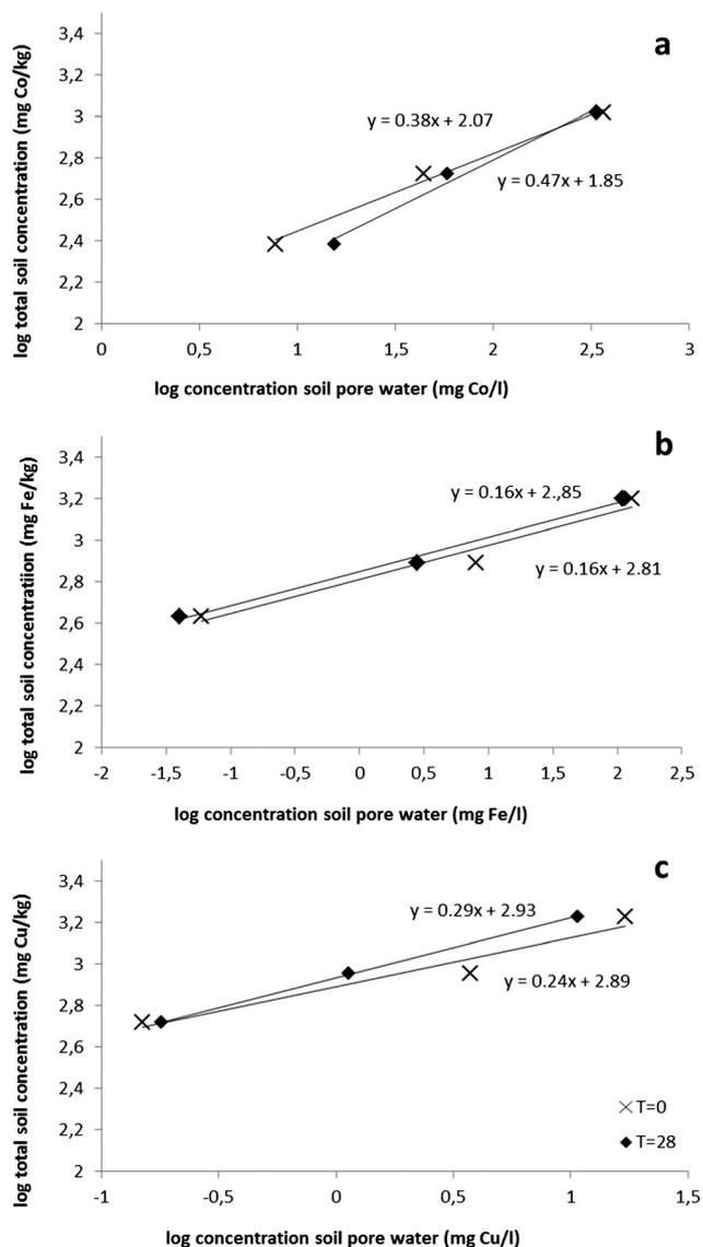
Fig. 1 Measured total metal concentrations in soil as a function of metal concentrations in soil pore water. Lines and equations represent the fit of the Freundlich isotherm to the data for the sorption of Co (panel a, CoCl<sub>2</sub>), Fe (panel b, FeCl<sub>3</sub>) and Cu (panel c, CuCl<sub>2</sub>) in spiked Lufa 2.2 soil at  $T = 0$  (X) and  $T = 28$  days (♦).
