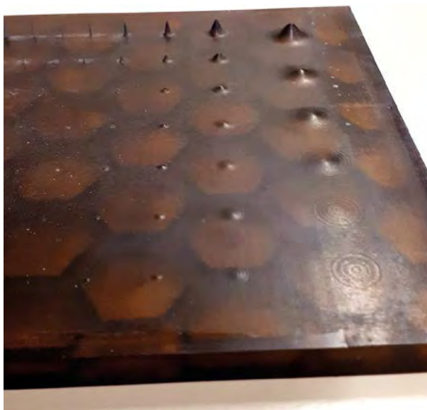
Figure 6. Photo of the 3D printed lesion phantom to quantify the errors induced by using the optical scanner and the analysis tool. The lesion phantom contains Gaussian shaped lesions ranging from 0.1 to 5 mm in elevation and 0.5 to 16 mm in diameter.
