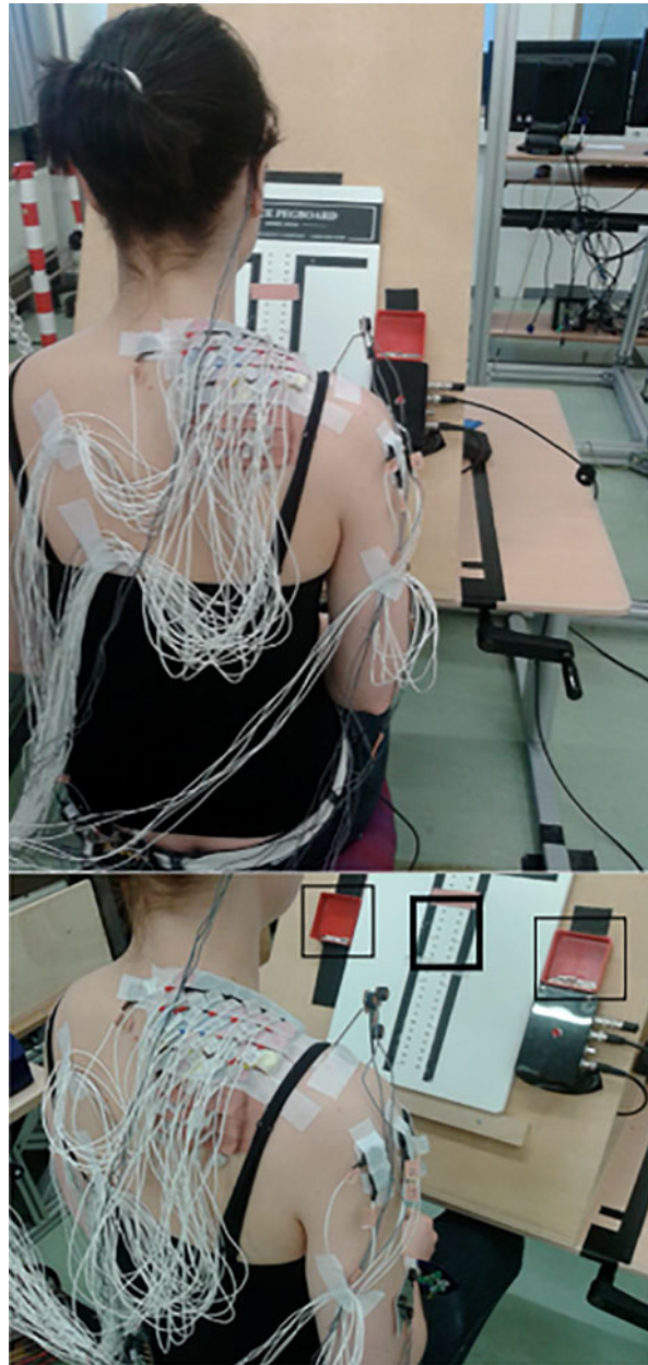
Figure 1. A sample subject performing the Pegboard task. Holes were bimanually filled and emptied with pins (1.3 g) from and to the two bins next to the Pegboard (see the two thin rectangles). A restricted part of the Pegboard was used ( 6 \times 2 matrix, see the thick rectangle) to keep the task as static as possible. At the right shoulder (M. Trapezius), muscle activity is measured using two grids of electrodes.
