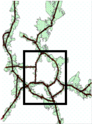
Figure 3: Selected cells covering the highways of Amsterdam and its surroundings Note 1: The Greater Amsterdam area within the black rectangle contains 122 GSM zones. Note 2: 109 of these GSM zones have an area coverage of > 70% of the highways.
