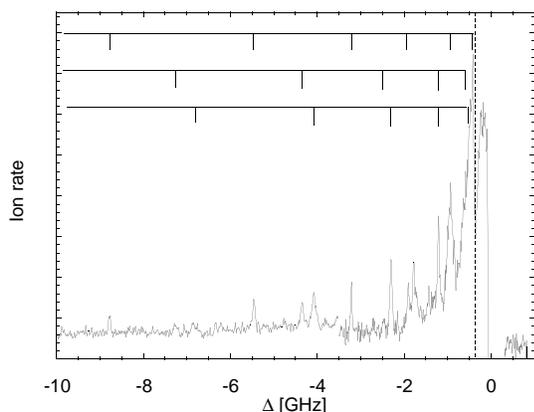
FIG. 2. Photoassociation spectrum of  $\text{He}^*$  as a function of the detuning  $\Delta$  of the probe laser. For the left side of the spectrum (from  $-10$  to  $-3.5$  GHz) the probe laser intensity is  $1.2 \times 10^5 I_{\text{sat}}$  and for the right side (from  $-3.5$  to  $0$  GHz)  $7.5 \times 10^4 I_{\text{sat}}$ . The assignment of the states to vibrational series is shown on top.
