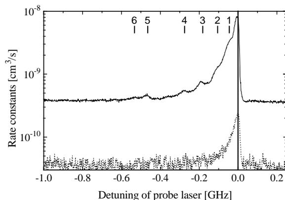
FIG. 1. Rate constants for ionization (solid line) and for radiative escape (dashed line). Both are measured with circularly polarized light. The radiative escape signal for  $\Delta < -0.25 \text{ GHz}$  and  $\Delta > 0.020 \text{ GHz}$  is a constant background of slow atoms released during the trapping phase against which the signal of the faster atoms is measured.
