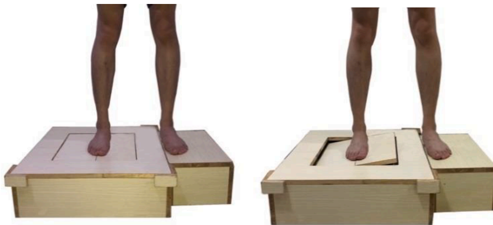
Fig. 1. Depict of ankle proprioceptive accuracy measurement using the Active Movement Extent Discrimination Apparatus (AMEDA). The left picture illustrates the horizontal start position, the right picture illustrates one of the four inversion angles.
