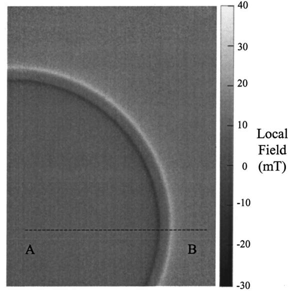
FIG. 1. Local field map obtained from MO-ILIA (see text) magneto-optical imaging of ring 2 (125  $\mu\text{m}$  width), with an applied field of 8 mT, at  $T=4.2$  K. The scale bar gives the local field values in mT. We observe a positive bright outline at the outer edge of the ring, while a negative dark outline is visible at the inner edge of the ring. The profiles shown in Figs. 3(a) and 6(a) are measured along the dashed line  $AB$ .
