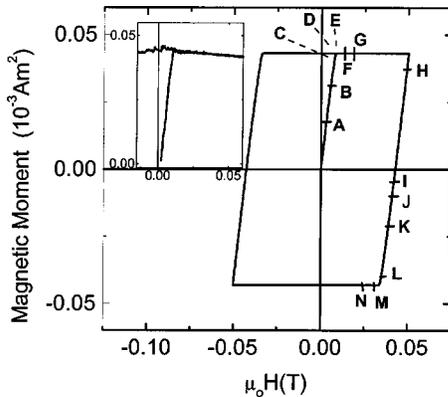
FIG. 5. Calculated hysteresis loop starting from ZFC conditions. The characters refer to the curves in Fig. 3 ( $A-G$ ) and Fig. 6 ( $H-N$ ). Inset: part of the experimental magnetization loop from torque measurements. The letters refer to the curves in Fig. 3(a) ( $A-G$ ).
