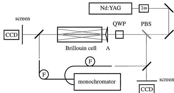
Fig. 1. Scheme of the experimental setup: PBS, polarization beam splitter; QWP, quarter-wave plate; A,  $2.5^\circ$  quartz axicon; CCD, CCD camera for beam-profile recording; F's, bare-tip single-mode fibers. A double fiber-input monochromator is used for frequency measurements.
