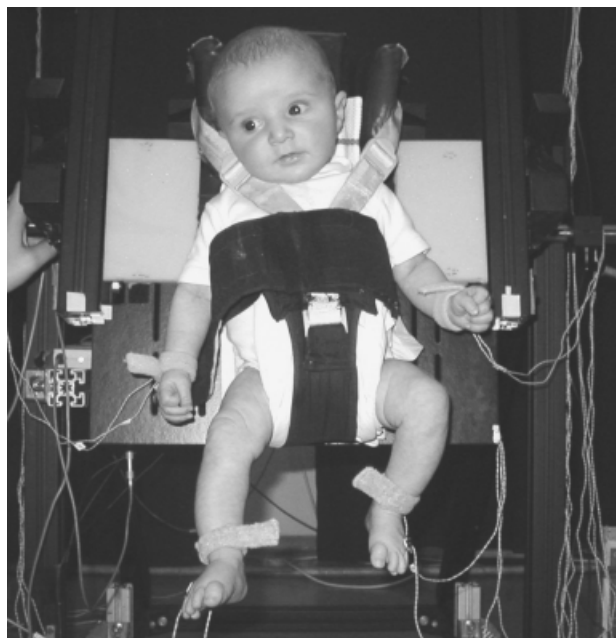
Figure 1. One volunteer positioned vertically in the seat within the laboratory. Infants had their trunks secured but had freedom of movement of their arms and legs. The seat also rotated to position infants horizontally.
