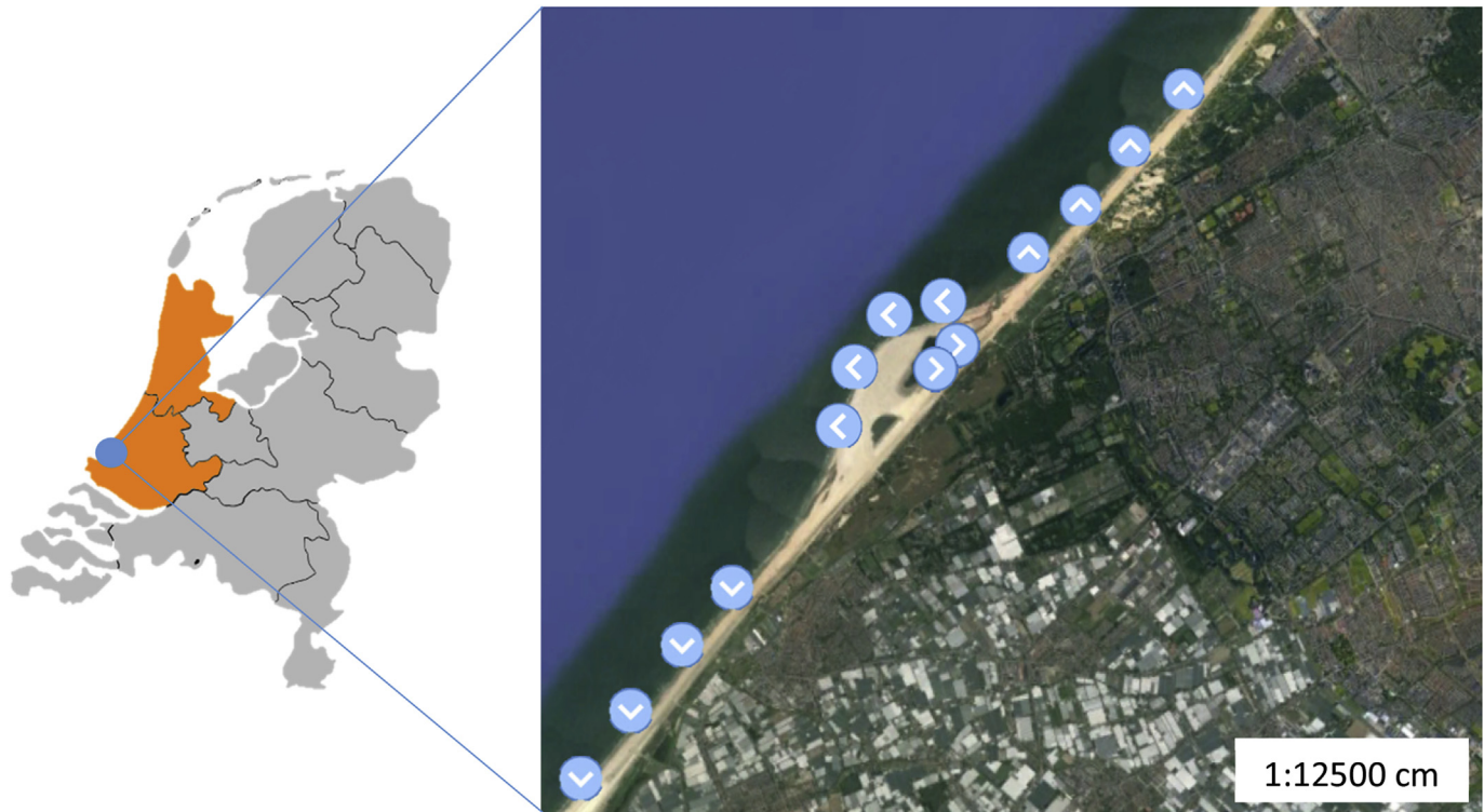
Fig. 1. Map of the Netherlands with the position of the ‘Sand Motor’ mega-nourishment (blue dot) and the region in which all other beaches of the combined data set were located (orange provinces). A satellite image of the mega-nourishment area (right) with the transects at the hook (arrow left), north (arrow up), south (arrow down) and in the lagoon (arrow right) of the mega-nourishment indicated. (For interpretation of the references to colour in this figure legend, the reader is referred to the Web version of this article.)
