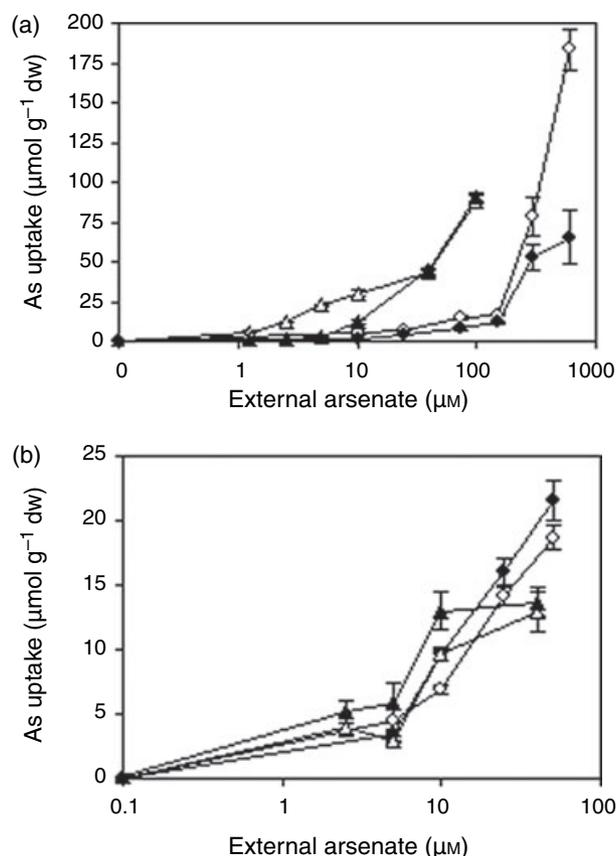
**Figure 2.** Plant arsenic uptake ( $\mu$ mol g<sup>-1</sup> root dw) of *Holcus lanatus* (mean SE,  $n = 5$ ) exposed to (a) arsenate [As(V)] and (b) arsenite [As(III)] for 5 days. Non-metallicolous (NM; triangle) and metallicolous (M; circle) plants at 10 (open symbols) and 100  $\mu$ M P supply (closed symbols) are presented.
