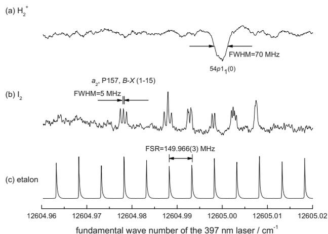
FIG. 3. Spectrum showing the transition from the  $EF\ ^1\Sigma_g^+(v=0, N=1)$  level to the  $54p1_1(0)$  level (a) with the  $I_2$  calibration (b) and etalon (c) traces. The position of the  $a_2$  hyperfine component of the P157,  $B-X$  (1–15) rovibronic transition of  $I_2$  was determined to be at 377 886 781.37(10) MHz using a frequency comb.
