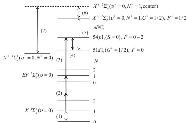
FIG. 1. Schematic energy level diagram of  $H_2$  illustrating the procedure used to determine the ionization energy of  $H_2$ . The energy intervals are not to scale. The bold arrows show the multiphoton excitation scheme used in the present experiment.
