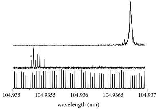
FIG. 1. Recording of the  $R(0)$  line in the  $B-X$  (4,0) Lyman band with the  $I_2$  reference spectrum and etalon markers for the calibration. The line marked with \* is the  $t$ -hyperfine component of the  $R(80)$  line in the  $B-X$  (9,4) band of  $I_2$ .
