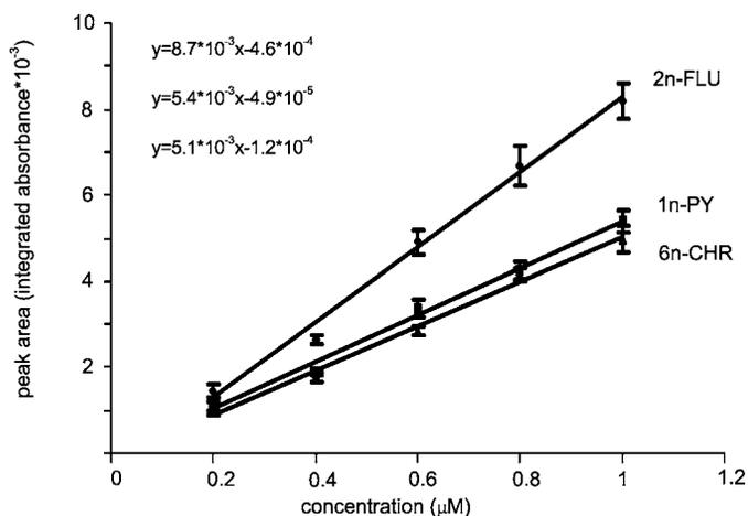
FIG. 7. Calibration curves of 2-nitrofluorene, 1-nitropyrene, and 6-nitrochrysenes show that CRDS detection is linear up to at least 200 ppb. Each concentration was measured three times; the error bars show the standard deviation.  $R^2$  values of the regression lines are 99.2%.
