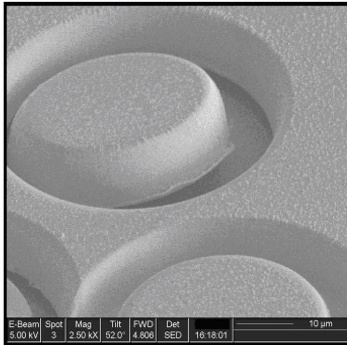
**Figure 7.** LiNbO<sub>3</sub> disks fabricated by crystal ion slicing and FIB sculpting.
