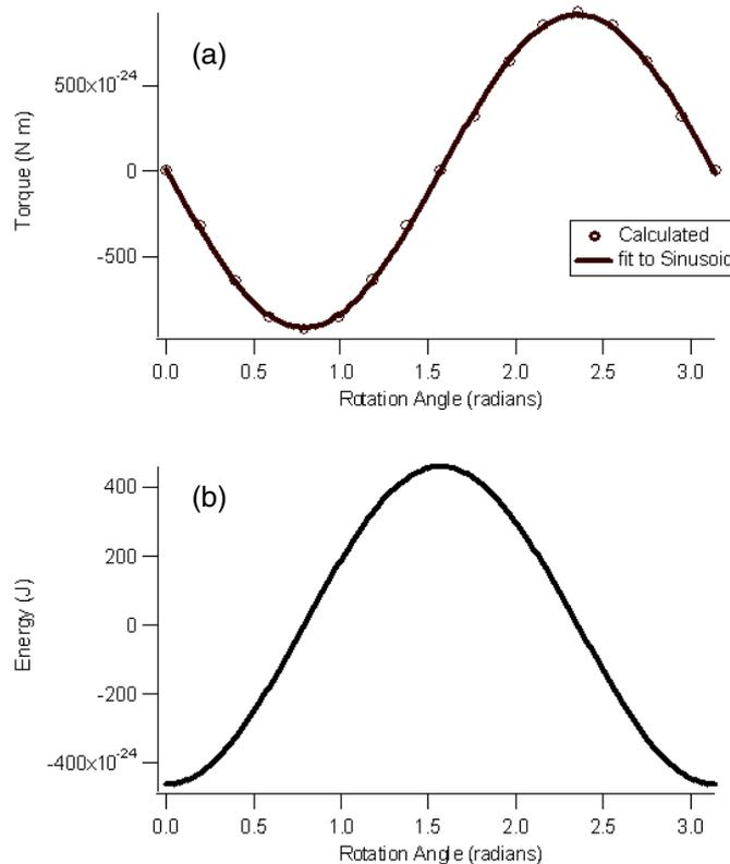
**Figure 2.** Calculations of the QED torque and energy between a  $\text{LiNbO}_3$  disk and a calcite plate. (a) Calculated torque ( $\circ$ ) and sinusoidal fit (line). (b) Calculated energy from sine fit of panel (a).
