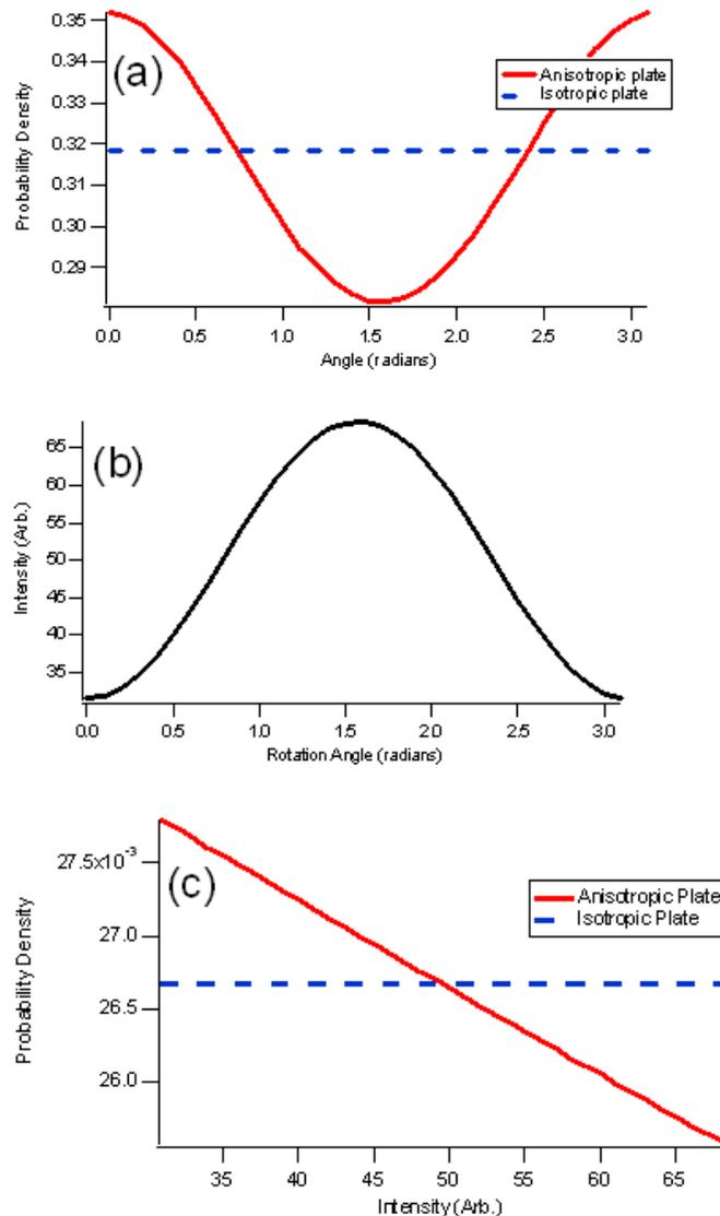
**Figure 5.** Probability distributions. (a) Probability of detecting a rotation  $\theta$ . (b) Intensity transmitted through the experimental set-up as a function of  $\theta$ . (c) Probability as a function of recorded intensity.
