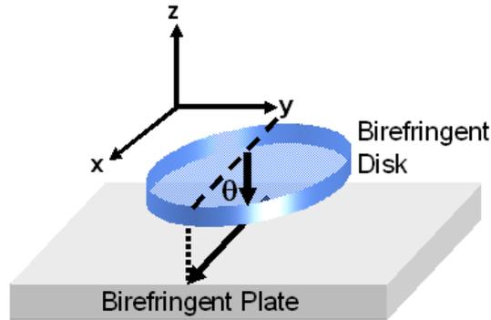
**Figure 1.** Schematic of the system under investigation. Two birefringent plates with in-plane optical anisotropy are placed at close proximity with angle  $\theta$  between their optical axes.
