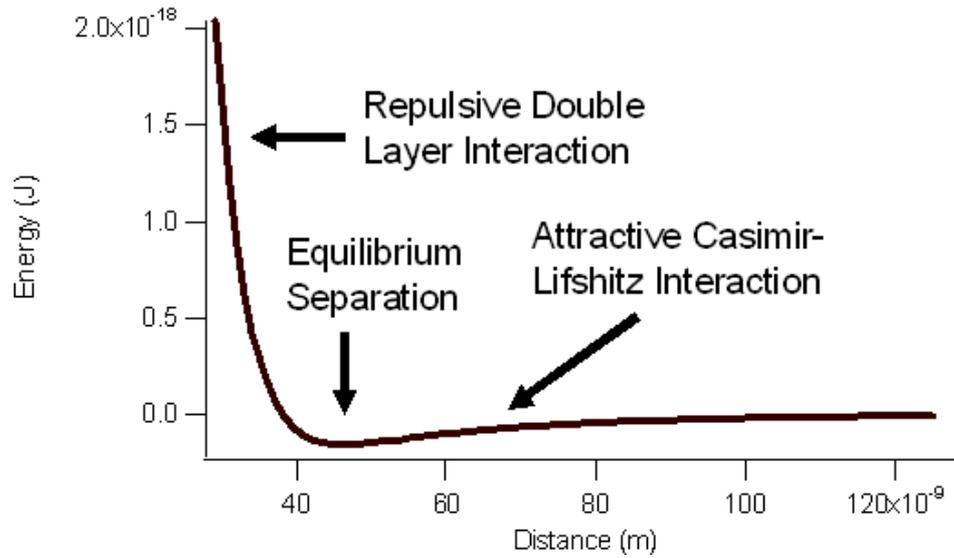
**Figure 3.** Energy as a function of separation between a  $\text{LiNbO}_3$  disk and a calcite plate including contributions from the double layer interaction (dominant at close range), the Casimir–Lifshitz interaction (dominant at longer range) and gravity (negligible). Equilibrium is obtained around 50 nm.
