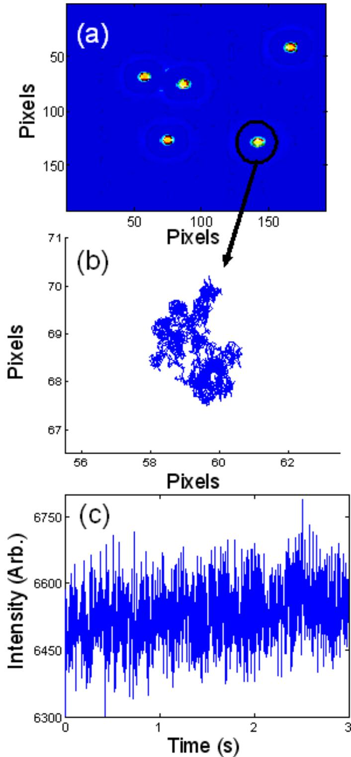
**Figure 6.** Computerized tracking and intensity fluctuations for  $10\ \mu\text{m}$  polystyrene spheres from early calibration procedures. (a) CCD image and determination of particle centres. (b) Tracking of one sphere over 5 s. (c) Intensity fluctuations of scattered light.
