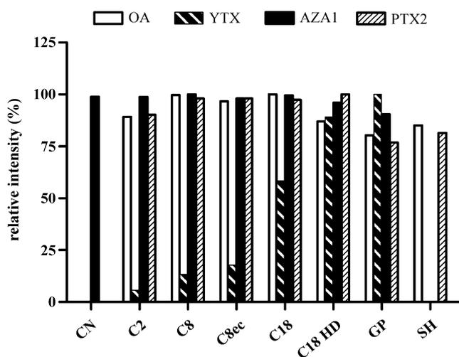
**Fig. 4** Sorbent screening using the Symbiosis Pharma automated SPE system. Highest signal intensity per individual toxin set at 100%. Wash with 20%  $v v^{-1}$  methanol/water elution with 1%  $v v^{-1}$  NH<sub>4</sub>OH in methanol
