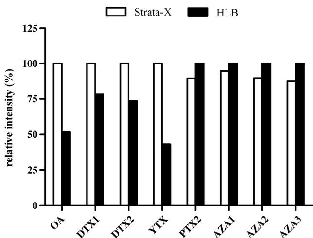
**Fig. 5** Relative intensity of selected toxins on two different sorbents with the preliminary SPE protocol. Highest intensity per individual toxin is set at 100%. Wash with 50%  $v v^{-1}$  methanol and elution with methanol
