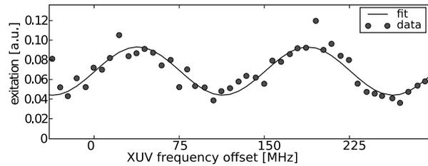
Fig. 6. Direct XUV comb excitation ion signal on the helium  $1s^2 \ ^1S_0 - 1s5p \ ^1P_1$  transition at 51.6 nm, where  $f_{rep}=148$  MHz, and a mixture of helium and neon was used. The zero of the frequency axis is based on theoretical level energies from Ref.<sup>10</sup>
