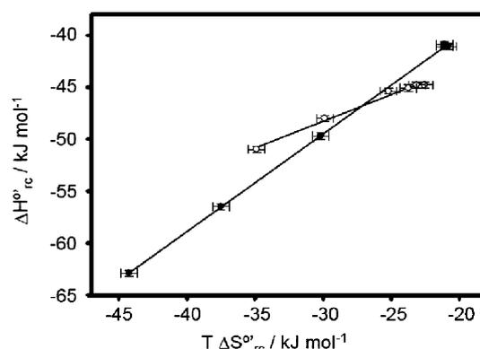
**Fig. 4** Enthalpy–entropy compensation plots at different urea concentrations for the reduction thermodynamics of the B1 states of ycc (filled circles) and K72AK73AK79A (open circles) immobilised on an MUA/MU-modified gold electrode at 293 K. The solution contained 5 mM sodium perchlorate and 5 mM phosphate buffer (pH 7). The straight lines represent the least-squares fits to the data, yielding a slope of 0.94 and 0.51 for ycc and K72AK73AK79A, respectively
