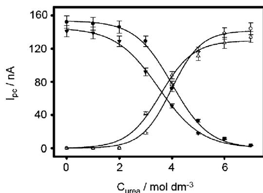
**Fig. 2** Cathodic peak currents measured for *ycc* and its variant K72AK73AK79A immobilised on an MUA/MU-modified gold electrode at different urea concentrations. *ycc*, wave I filled circles; *ycc*, wave II open circles; K72AK73AK79A, wave I inverted triangles; K72AK73AK79A, wave II upright triangles. The solution contained 5 mM sodium perchlorate and 5 mM phosphate buffer (pH 7,  $T = 278$  K)
