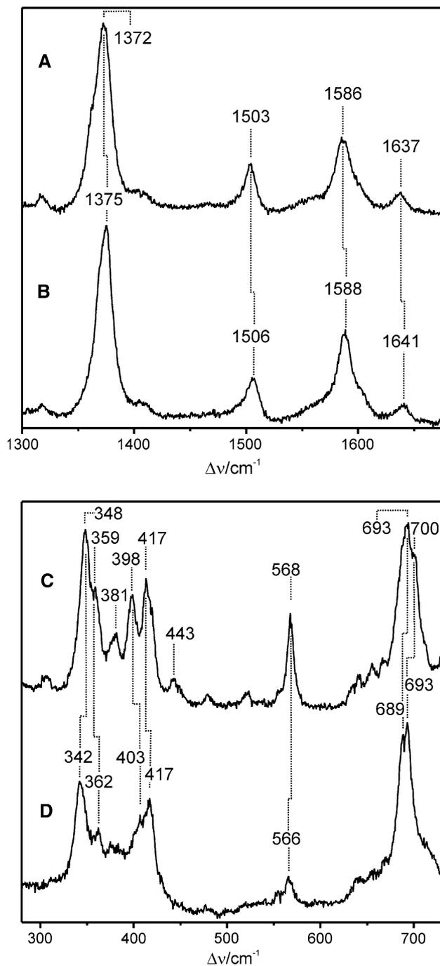
**Fig. 3** Surface enhanced resonance Raman spectra of ycc immobilised on an MUA/MU-coated silver electrode at +0.1 V (vs. the saturated calomel electrode) in the absence of urea in the electrolyte solution (A, C) and in the presence of 8 M urea (B, D). The solution contained 5 mM sodium perchlorate and 5 mM phosphate buffer (pH 7,  $T = 278$  K). The spectra were obtained with 413-nm excitation
