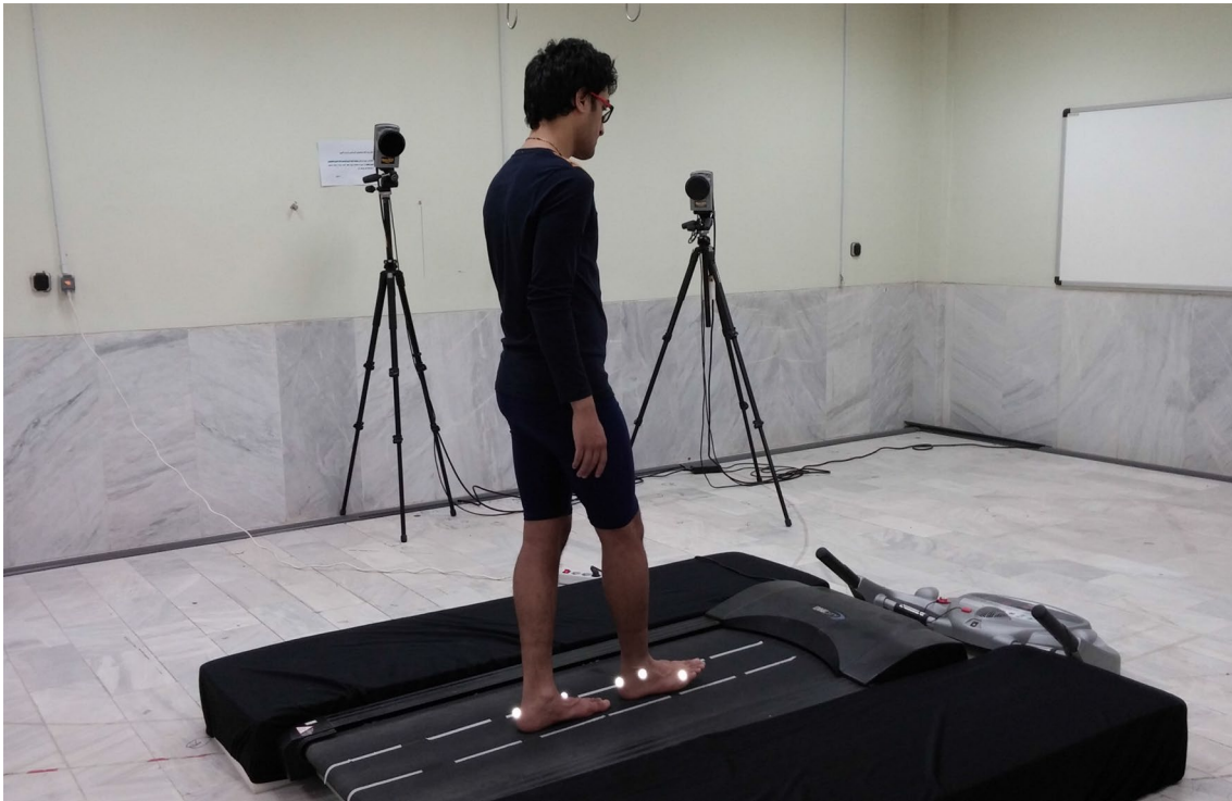
Fig. 1 Experimental set-up: walking within the narrow path traced using tape on the treadmill belt. The distance between the two lines is adjusted to 50 % of the distance between the participant's anterior superior iliac spines
