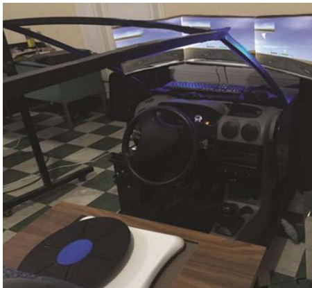
Figure 1 — The driving simulator and overview of the experimental setup in unstable sitting surface conditions.
