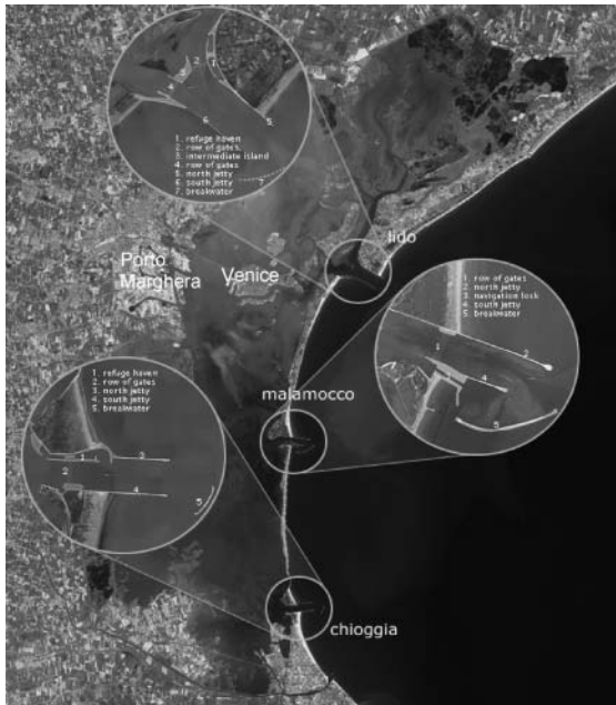
Figure 6. Project design of the mobile barrier system to protect Venice from flooding (MOSE). Source: CVN 2010.
