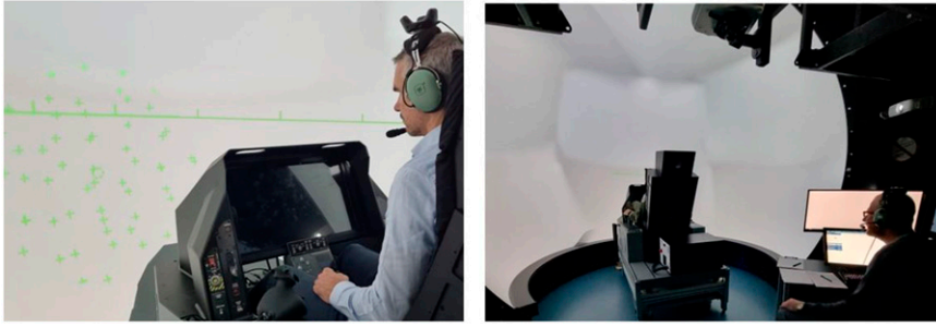
Figure 1. Experimental setup. A pilot in the fixed-base flight simulator countering the roll disturbance with the stick (visually indicated by the horizon line, which spanned the whole outside world) while actively aiming his head (small dotted circle) on the moving visual target, as projected in the dome.
