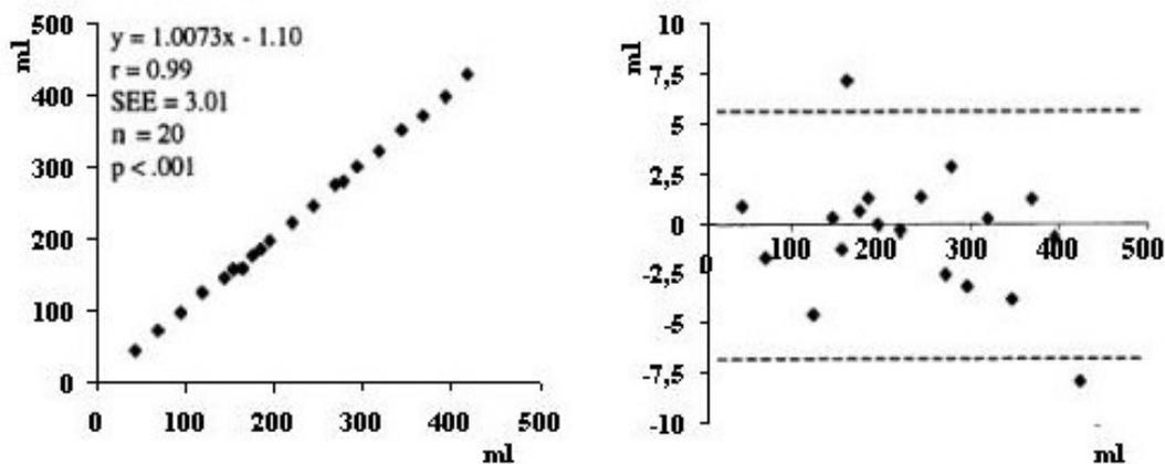
Linear regression (A) and Bland-Altman plot (B) of true balloon volumes versus 3D balloon volumes. Linear regression equation, its coefficient  $r$ , and standard error of estimate (SEE) are shown, as well as number of observations ( $n$ ). In Bland-Altman plot, bias and 95% confidence limits are indicated.
