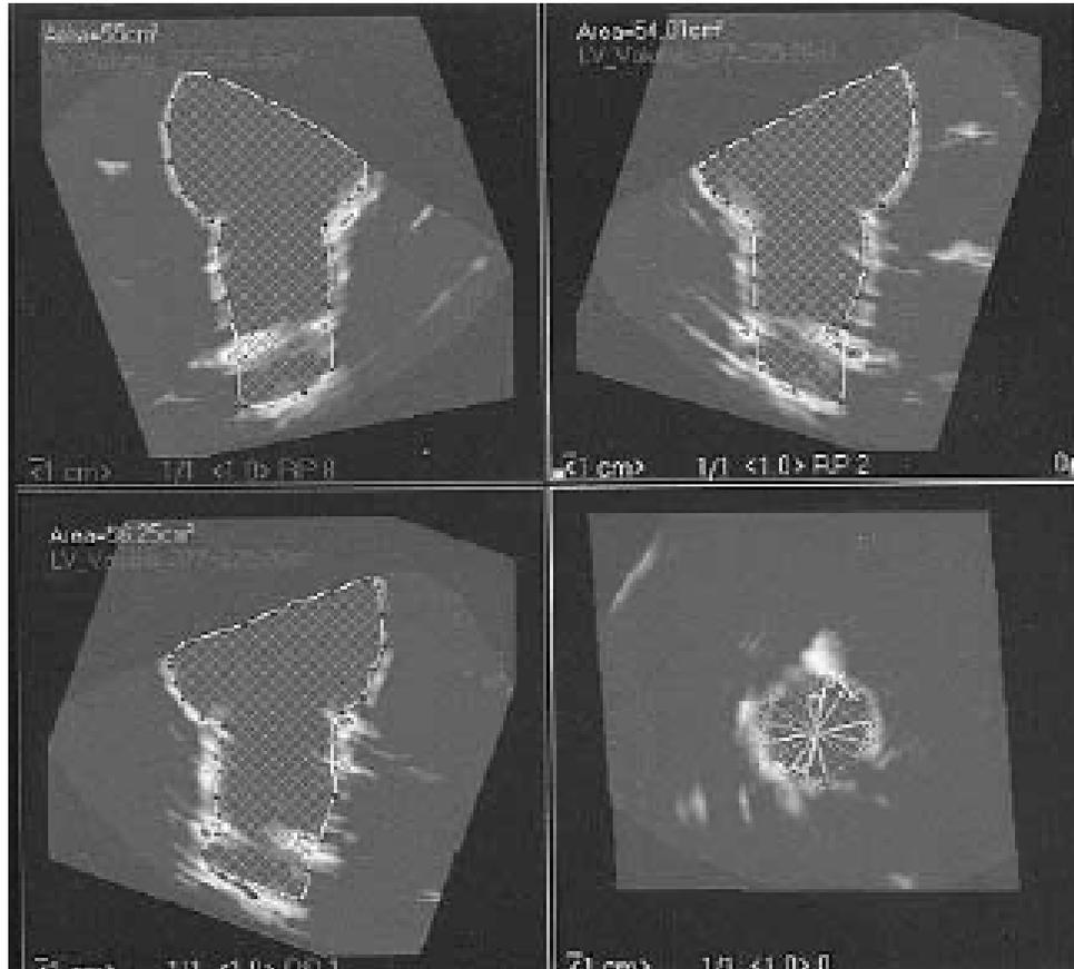
3D analysis of aneurysmatic 350-mL balloon with 10-degree angulation and 5.3-cm transducer tip distance. Note how sector cuts off a substantial part of balloon so that true volume of 350 mL was reduced to measured volume of 225 mL. Three long-axis planes and one short-axis plane are shown.
