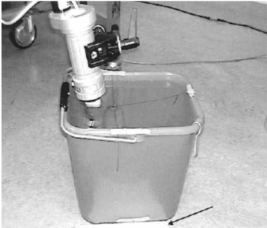
Experimental setup used in balloon models and autopsy hearts is shown with water bath, flexible mechanical arm, transducer, and centimeter scale attached to floor (arrow), along which the water bath was displaced.
