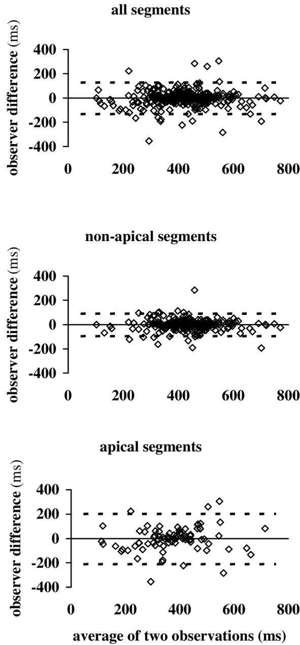
Bland-Altman plots of the reproducibility of timing. The horizontal axis is the average of 2 measurements and the vertical axis the difference between the first and second measurements of 1 observer (in milliseconds). Dashed lines, the 95% confidence interval. (top) The reproducibility of all segments, (center) the reproducibility of non-apical segments, and (bottom) the reproducibility of apical segments. The reproducibility of nonapical (vs apical) segments was significantly better.
