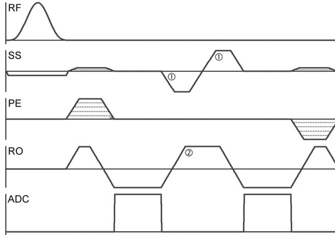
Figure 2.1: Multiecho PC-SSFP sequence. The bipolar gradient ① is placed on the slice-select axis (SS) at the time interval between the two readouts for through-plane flow encoding. The readout axis (RO) contains the gradients for the two echoes and the fly-back gradient ② is placed between them.
