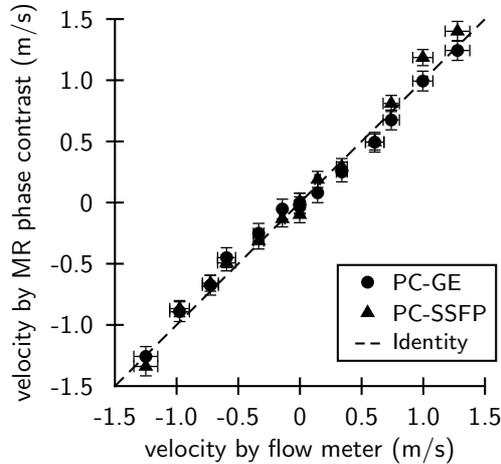
Figure 2.2: *In vitro* validation: cross sectional averaged velocity measured with PC-SSFP and PC-GE against flow meter readings. Error bars indicate the estimated measurement error. Data were consistent with the line of identity (PC-SSFP: slope 1.03  $P=0.4$ , offset 0.03 m/s  $P=0.3$ , PC-GE: slope 0.94  $P=0.03$ , offset 0.0 m/s  $P=0.8$ ), and the residual errors were small (RMS 0.1 m/s for PC-SSFP and 0.05 m/s for PC-GE).
