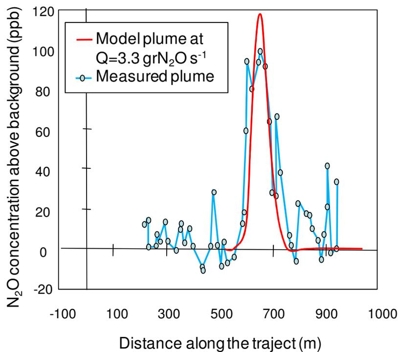
Figure 5.4 The N<sub>2</sub>O plume measured at the transect together with the modelled plume.
