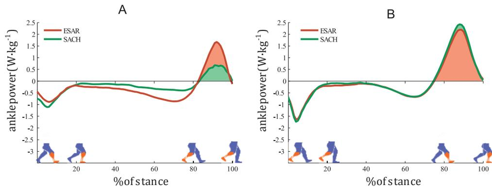
**Figure 2. Push-off power over the stance period.**
