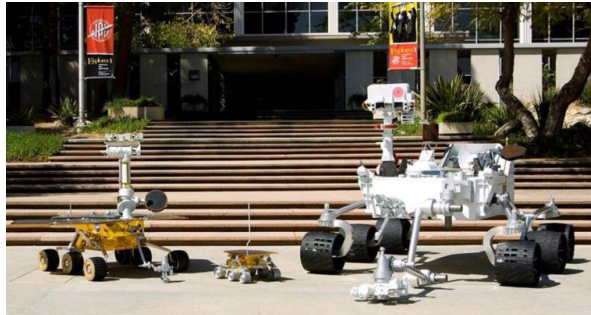
Figure 1.8. Comparison of the Mars Exploration Rovers (MER) robot (Spirit and Opportunity left) with the robot Pathfinder (Sojourner, centre) and the Mars Science Laboratory robot (Curiosity, right) (Credit: Jet Propulsion Laboratory (JPL))
