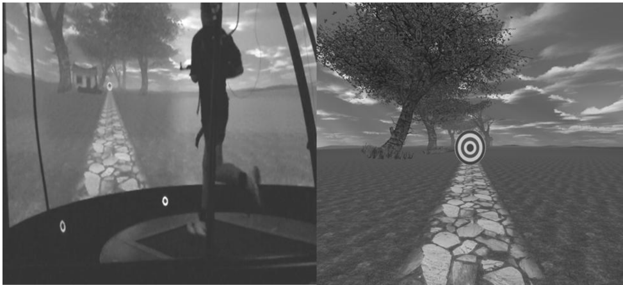
Figure 4.2. (a) Photo of the CAREN system with the treadmill (embedded in the platform) and the projection screen. (b) Virtual environment including the round shaped target.
