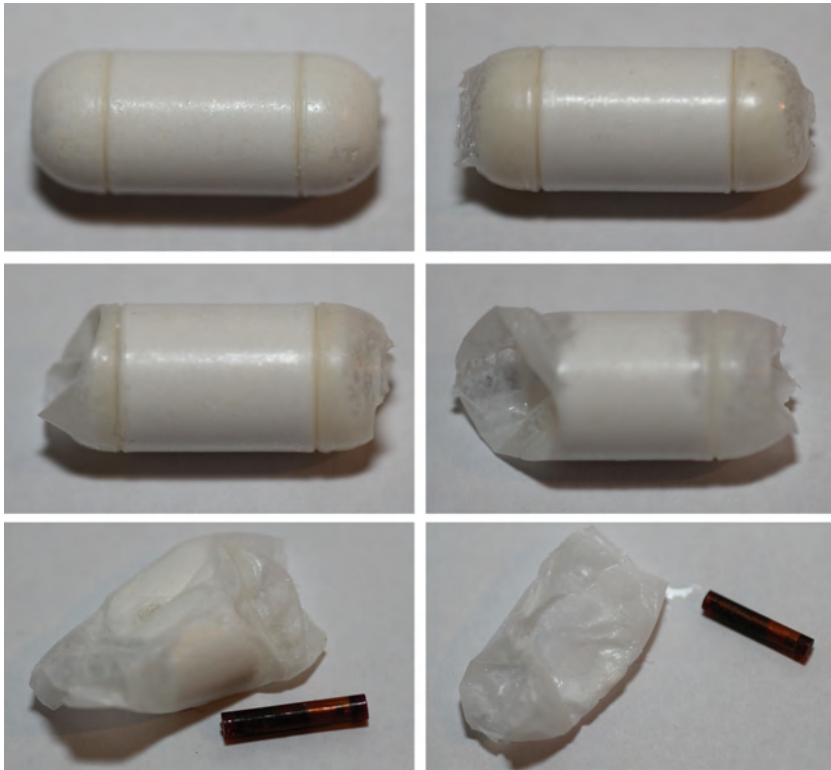
Figure 5.7: Photographic sequence of the consecutive stages of a dissolving patency capsule. The timer plugs can be seen at both ends of the capsule. When these dissolve, the capsule disintegrates. The small radiofrequency identification tag that is originally located in the middle of the capsule can be seen at the lower images. The flexible plastic sleeve can pass even tight strictures.
