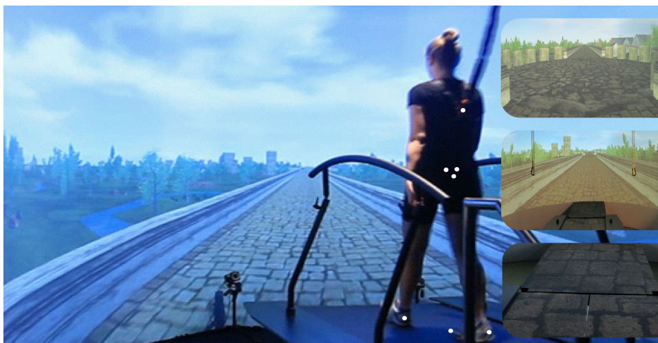
Fig 8-1. GRAIL experimental set-up, consisting of a dual-belt treadmill, 180° VR environment with ground projection (see inset) and optoelectronic motion analysis system. The speed-matched scene consisted of a simple road with a changing rural landscape.
