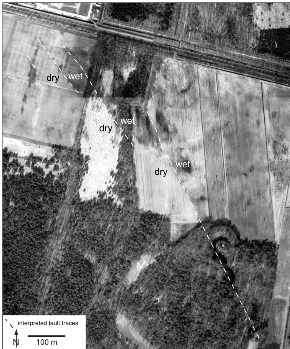
Figure 2.4: Aerial photograph of the Gilze-Rijen Fault as it crosses farming land near the city of Tilburg (with permission of the municipality of Tilburg). The fault clearly separates different hydrologic units; for location see Figure 2.14.
