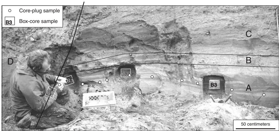
Figure 3.5: The wall of the trench over the Geleen Fault during sampling of box cores and core plugs.
