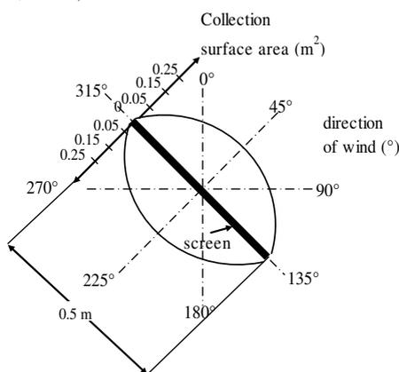
Figure IV.4. 2-D screen fog collector (0.5 x 0.5 m) oriented to NE (45°) and the theoretical relationship between effective collection surface area (from 0 to its maximum 0.25 m<sup>2</sup>) and wind direction (°).
