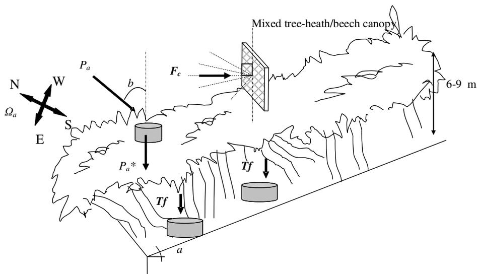
Figure IV.3. Measurement of water inputs at canopy and soil surface levels in a hillcrest tree-heath forest oriented towards the NE ( $\Omega_a$ ) on a 25% slope ( $a$ ).  $P_a$ : meteorological rainfall (corrected for wind loss around the gauge);  $P_a^*$ : rainfall corrected for topographic and wind effects (hydrological rainfall);  $b$ : angle of the rainfall;  $F_c$ : wind-direction corrected fog water volume;  $T_f$ : throughfall.
