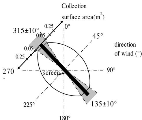
Figure IV.5. 2-D screen fog collector (0.5 x 0.5 m) oriented to NE ( $45^\circ$ ), the theoretical relationship between effective collection surface area and wind direction ( $^\circ$ ) and the adopted spectra ( $135 \pm 10^\circ$  and  $315 \pm 10^\circ$ ) in which the effective screen area is assumed to be constant ( $0.04 \text{ m}^2$ ).
