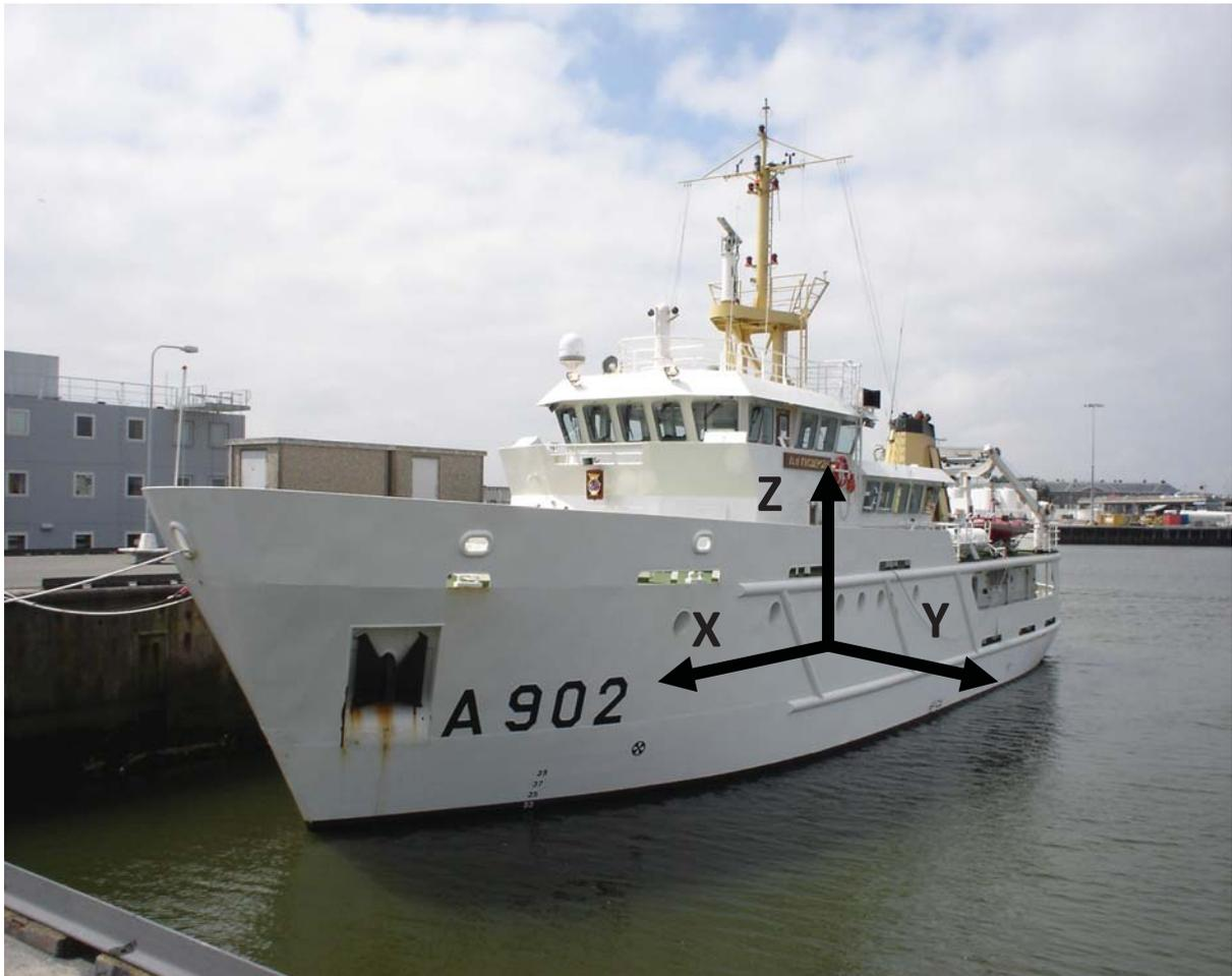
**Figure 4-1.** Photograph of the Royal Netherlands Navy training vessel “Van Kinsbergen” on which the experiment took place. The local coordinate system of the ship, which was used in the present study, is indicated.
