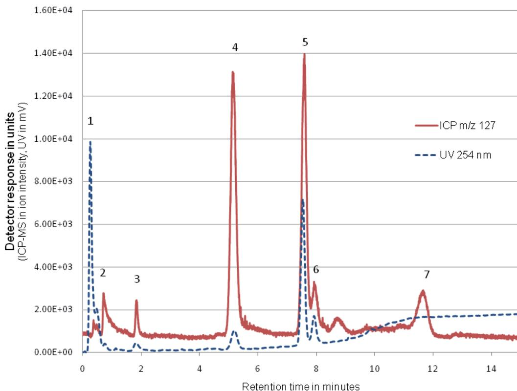
**Figure 7:** Overlay of HTLC-ICP-MS (solid) and HTLC-UV (dashed) chromatogram of the electrochemical oxidation products of SB-I.
