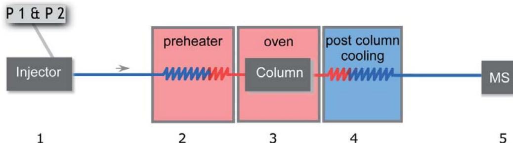
**Figure 1:** Schematic representation of the HTLC-MS setup with, (1) Injector and gradient pumps, (2) Solvent preheating compartment, (3) Column heating block, (4) Post column cooling unit and (5) ICP-MS or ESI-MS.
