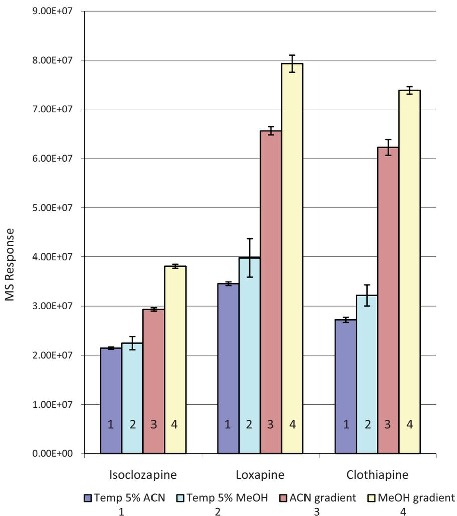
**Figure 2:** Comparison of ESI-MS peak areas (arbitrary units) of standards with temperature and organic solvent gradients.
