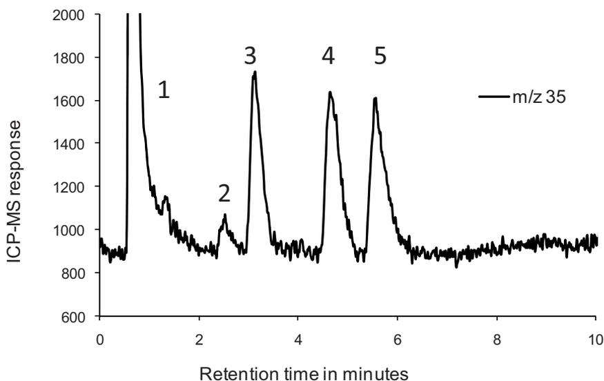
**Figure 3:** HTLC-ICP-MS chromatogram for chlorine ( $m/z$  35) in a 250  $\mu\text{M}$  standard mix of iso-clozapine, loxapine and clothiapine using 5% ACN 0.2 % FA as mobile phase. (1) polyatomic interference of  $^{34}\text{S}+\text{H}$ ; (2) Chlorine containing impurity with  $m/z$  355.1325; (3) isoclozapine; (4) loxapine; (5) clothiapine.
