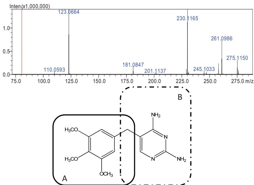
**Figure 1:** ESI-MS-MS spectrum of Trimethoprim and fragmentation of Trimethoprim in two parts (A  $m/z$  181 and B  $m/z$  123) indicating site of modification in the metabolites.
