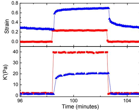
**Figure 5.4** – (Color online) Close-up of the strain and differential modulus  $K'$  during the 13<sup>th</sup> prestress pulse of 2 Pa for actin with NeutrAvidin (red squares) and for actin with filamin (blue triangles).
