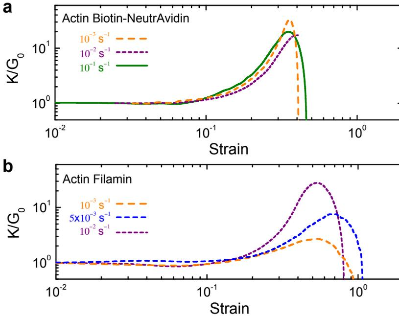
**Figure 5.2** – (Color online) Strain ramp protocol: The tangent modulus  $K = d\sigma/d\gamma$  normalized by the linear modulus  $G_0$  as a function of strain for various strain rates  $\dot{\gamma}$ :  $0.001 \text{ s}^{-1}$  (orange),  $0.005 \text{ s}^{-1}$  (blue),  $0.01 \text{ s}^{-1}$  (purple) and  $0.1 \text{ s}^{-1}$  (green). a) F-actin cross-linked with biotin-NeutrAvidin. b) F-actin cross-linked with filamin.
