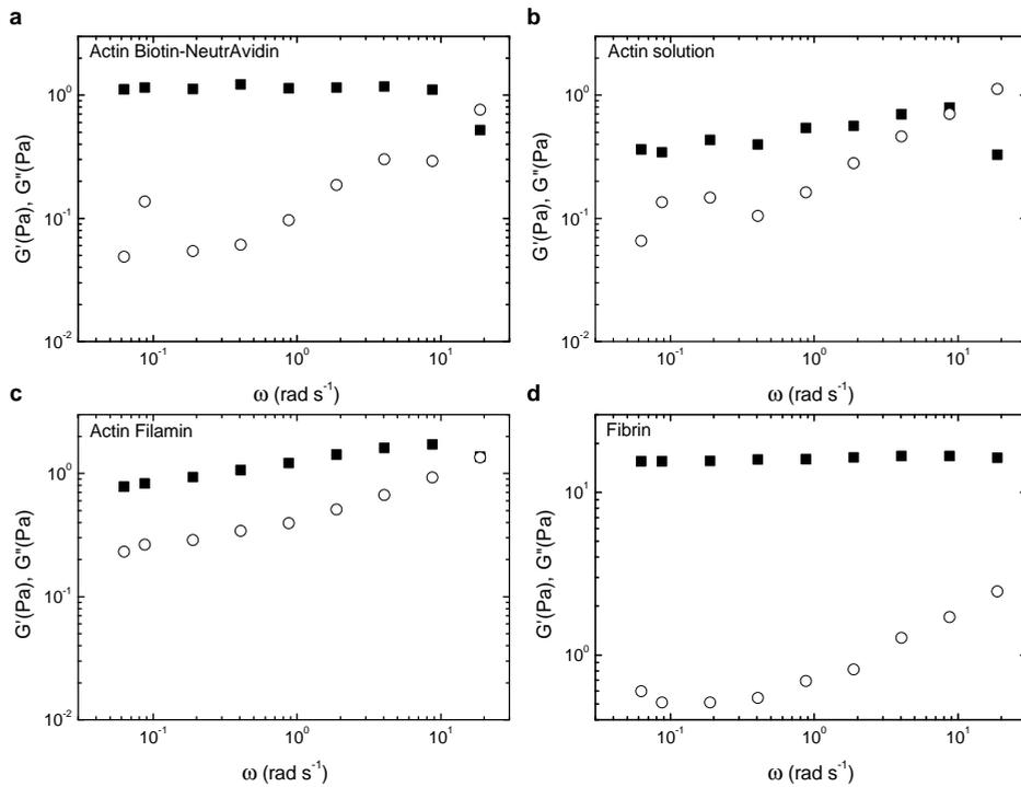
**Figure 5.1** – The linear viscoelastic moduli  $G'$  (squares),  $G''$  (circles) as a function of frequency for a) F-actin with a permanent biotin-NeutrAvidin cross-links. b) F-actin solution c) Actin cross-linked with the physiological linker protein filamin d) Fibrin with factor XIII.
