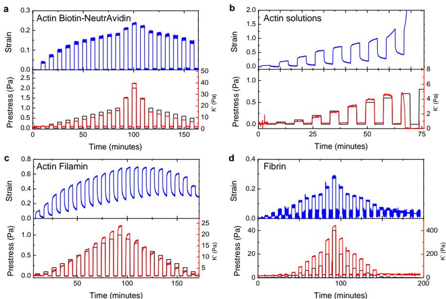
**Figure 5.3** – Prestress protocol: The strain (blue curves) and the differential modulus  $K'$  (red curves) as a function of time during 4 minute prestress pulses (black curves) applied every 4 minutes of increasing and then decreasing magnitude. a) F-actin with permanent biotin-NeutrAvidin cross-links. b) F-actin solution. c) Actin cross-linked with the physiological linker protein filamin. d) Fibrin with factor XIII.
