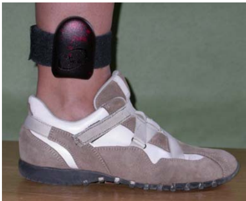
Figure 1. The StepWatch Activity Monitor 3 (SAM3, Cymatech Corporation, Seattle, WA, USA) is contoured to fit comfortably against the leg. An elastic attachment strap ensures that the monitor remains securely attached to the ankle without irritating the skin.
