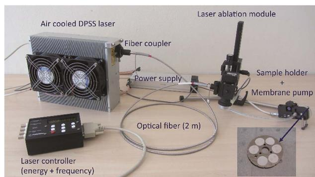
Fig. 1 Assembled portable laser ablation sampling device composed of a DPSS laser ( $\lambda$  532 nm), an optical fibre, a laser ablation module and a sample holder. Magnified inset image shows the sample wheel with six filters.
