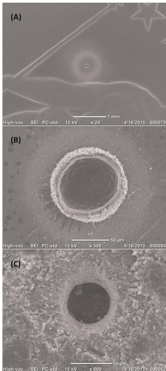
Fig. 2 SEM images of ablation pits generated with a tapered fibre; crater dimensions are  $\sim$ 60  $\mu\text{m}$  in width and depth. (A) and (B) craters in half a Swiss franc; note that the pale halo around the pit is debris which can be easily removed by cleaning with water. (C) Crater in a natural jadeite bearing rock from the Rio San Juan Complex in the Dominican Republic.<sup>15</sup>
