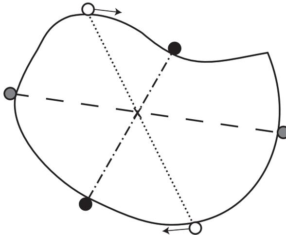
**FIGURE 8.1** An object with two possible opposition axes (dashed and dashed-dotted lines), and one set of grasping points (circles connected by dotted line) that will slip in the direction of the arrows if a grip force is applied and the friction is low
