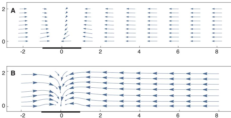
**FIGURE 8.3** (A) Example of a force field that is the combination of a repelling force perpendicular to the surface (2 cm wide) and an attractive force towards the grasping point at its center. (B) Possible resulting movement trajectories. This is a caricature of the fields used by Verheij et al. (2012) to model grasping trajectories
