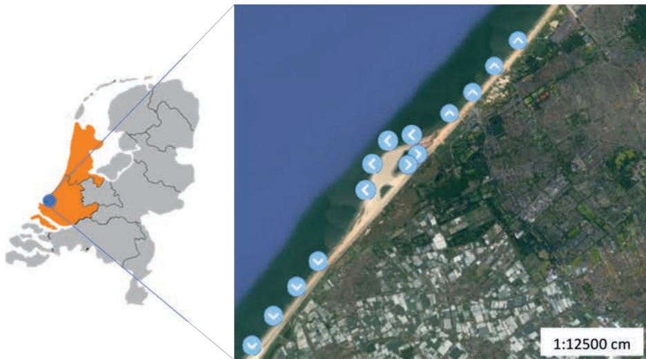
Figure 2.1 Map of the Netherlands with the position of the Sand Motor mega-nourishment (left: Large dot) and the region in which all other beaches of the combined data set were located (shaded provinces). A satellite image of the Sand Motor mega-nourishment area (right) with the transects at the hook (arrow left), north (arrow up), south (arrow down) and in the lagoon (arrow right) of the mega-nourishment indicated.
