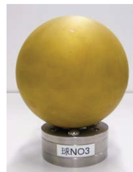
Fig. 2. Artefact: ball (Ø=120.0159 mm, sphericity=22.1 μm)
