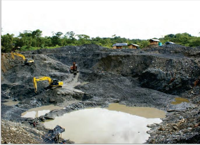
This is mining that uses mechanized equipment, such as small suction dredges, water pumps, sluice boxes, hydraulic excavators, and suction and spoon dredges. Photograph by Oro Verde.
