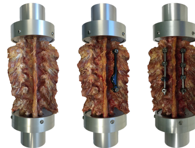
Figure 3. Biomechanical testing sequence with an untreated human cadaveric thoracic spine (left), after instrumentation with the posterior concave periapical nonfusion distraction device (middle), and after rigid pedicle screw-rod instrumentation (right).
