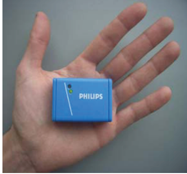
Figure 4-2: The wireless inertial sensor, which contains accelerometers, magnetometers and gyroscopes. Note that for the current study only the data from the accelerometers and gyroscopes were used.
